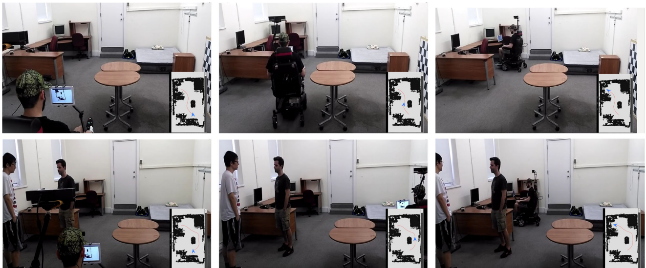
Fig. 14 Pictures from an experiment with the second subject. A static and a dynamic scene are shown at the top and bottom row respectively. The presence of people affect the subject's choice of paths, even though the people were not blocking any path
