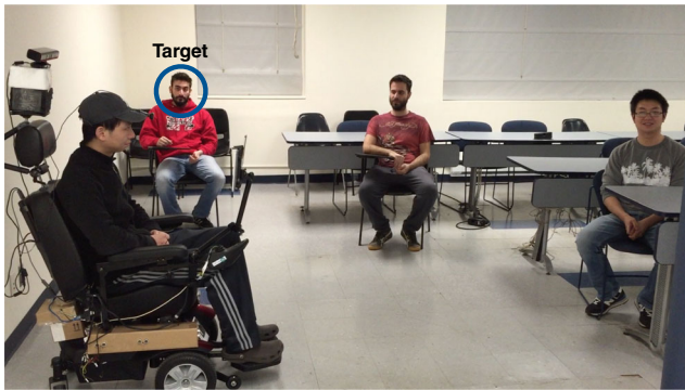
Fig. 16 An example of person-guided navigation. The user detects the person of interest to the left, which informs the wheelchair of the correct direction to turn. The face recognition task is then handed over from the egocentric camera to the RGB-D sensor
