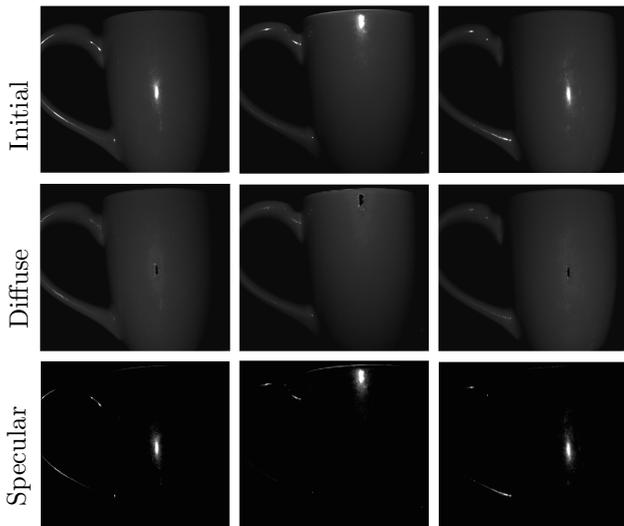
**Fig. 5** Test 2: Images of a painted ceramic cup before (first row) and after the reflection separation (second and third row).
