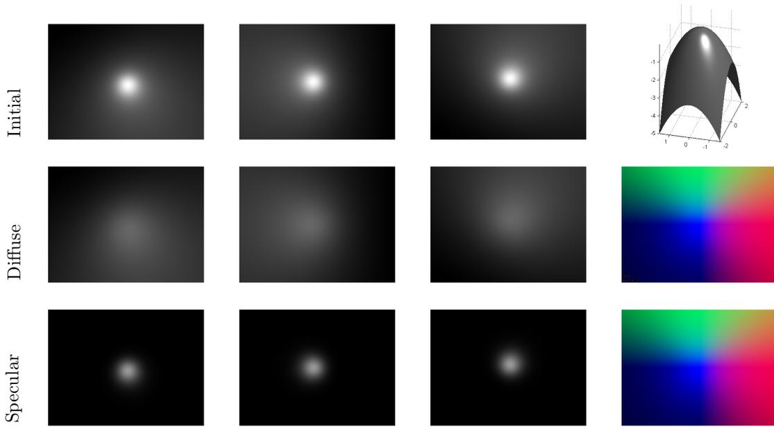
**Fig. 3** Test 1: Images of a paraboloid without noise before (first line) and after the reflection separation. In the last column: on the top, the original 3D shape. In the second and third rows are shown the color coded normal maps of the reconstructed shape using only the diffuse and the specular component, respectively.
