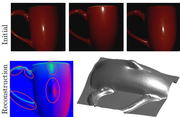
**Fig. 1** The top row shows three images of a painted ceramic cup. The bottom row shows the normal map where artifacts have been highlighted and the 3D shape reconstruction using traditional PS [37]. Bottom images show artifacts due to specular reflections.
