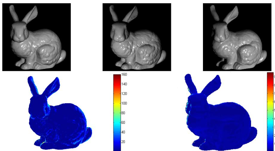
**Fig. 11** Test 6: The first row shows the 3 images used to reconstruct the bunny with our method. On the left second row, plot of the color coded normal error for the reconstructed surface using the algorithm in [16] and 10 images. On the right second row, the normal error when using our approach with only the 3 images.
