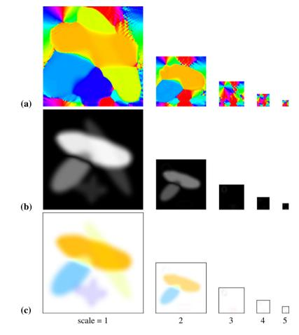
**Fig. 2** Synthetic overlapping texture: multiresolution monogenic signal analysis using Riesz–Laplace wavelets (five scales,  $\sigma = 1.5$ ) [69, 70]. **a** The local orientation is color-coded between  $-\frac{\pi}{2}$  and  $\frac{\pi}{2}$ . **b** The coherency (degree of directionality): isotropic features are dark and
