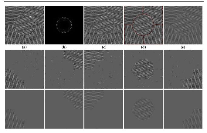
**Fig. 11** Simulated crystal lattice. 2D-SEG-VMD decomposition in two runs, first with, then without Lagrangian multipliers. See Sect. 7.6.3 in text for details and discussion. **a** Input image f. **b** Fourier spectrum  $\hat{f}$ . **c** First run reconstruction  $\sum_{k,i} A_k u_{ki}$ . **d** Partition (*red*) of second
