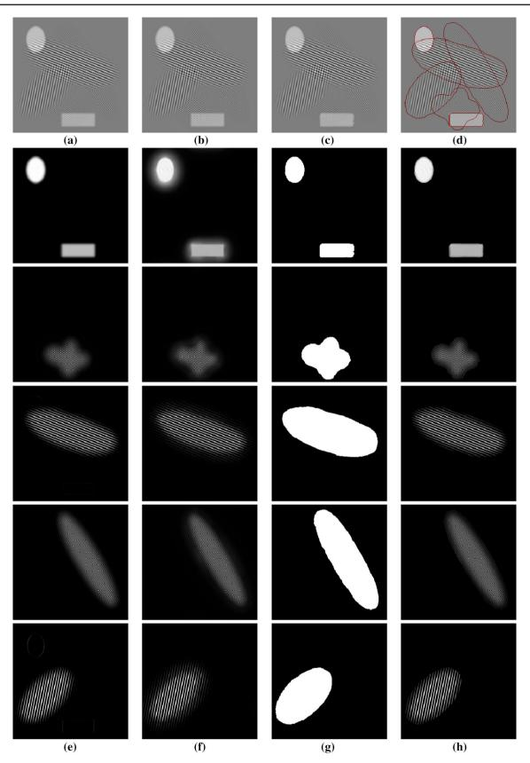
**Fig. 1** Synthetic overlapping texture **a** Input image f. **b** 2D-VMD reconstruction  $\sum_k u_k$ . **c** Compactly supported 2D-TV-VMD reconstruction  $\sum_k A_k u_k$ . **d** Support boundaries overlaid onto original image.
