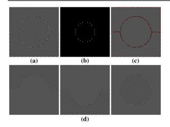
**Fig. 10** Three phases–three modes. **a** Input f. **b** Fourier spectrum  $\hat{f}$ . **c** 2D-SEG-VMD partition (*red*). **d** Phases  $A_k \sum_i u_{ki}$ . See Sect. 7.6.2 (Color figure online)
