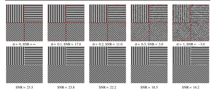
Fig. 5 Denoising. Top noisy f (noise SD  $\sigma$  and SNR) with detected phase borders (red). Bottom denoised signal  $\sum_k A_k u_k$ , SNR. See Sect. 7.3 (Color figure online)
