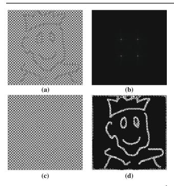
**Fig. 8** 2D-VMD inpainting. **a** Input image f. **b** Fourier spectrum  $\hat{f}$ . **c** Recovered modes  $\sum_{k} u_k$ . **d** Detected artifacts  $\chi$ . See Sect. 7.5
