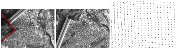
**Fig. 6** *First and last frames of the first robot sequence, and the dominant flow between frames 0 and 1 computed with TR model. The outlier area is framed in red in the first image.*
