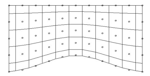
Figure 5.1: Convergent-divergent duct:  $\circ$  = nodes of primary cells, — = dual cells
