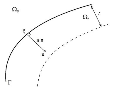
Figure 3: A local set of normal coordinates. Here  $\xi \in \Gamma$  is a point on the boundary, while s is the distance in the normal direction. A coordinate inside a neighborhood of  $\Omega_s$  has the form  $\mathbf{x} = \boldsymbol{\xi} + s \mathbf{n}(\boldsymbol{\xi})$ .
