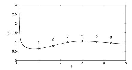
Figure 17: Drag versus time for RE = 550. Here  $\eta = 10^{-3}$ , N = 768, l = 0.05. Circles correspond to snapshots of the vorticity shown in figure 18.
