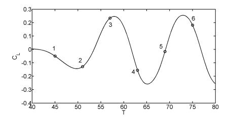
Figure 19: Lift versus time for the onset of the von Kármám street at RE = 550. The oscillations correspond to vortex shedding. Circles correspond to snapshots of the vorticity shown in figure 20.
