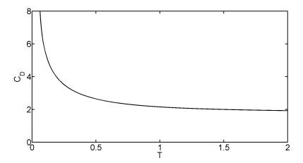
Figure 16: Drag versus time for RE = 40. Here  $\eta = 2 \times 10^{-4}$ , N = 512, l = 0.45.
