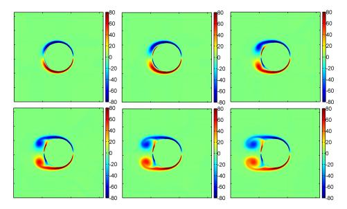
Figure 18: Snapshots of the vorticity for an impulsively started cylinder with RE = 550. Images are taken at times (l-r) T = 1, 1.66, 2.33, 3, 3.66, 4.33 and correspond to the circles in figure 17.
