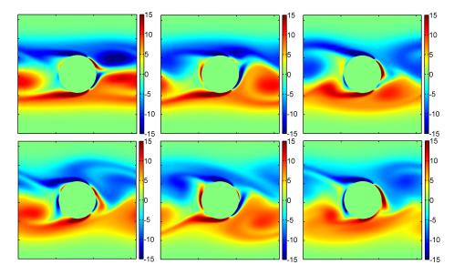
Figure 20: Snapshots of the vorticity for an impulsively started cylinder showing the onset of full vortex shedding and von Kármán type street [30]. Images are for RE = 550, and taken at times T=45,51,57,63,69,75 corresponding to the circles in figure 19.
