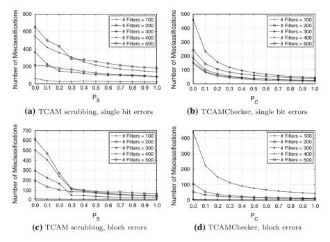
Fig. 5 Accuracy comparison of TCAM scrubbing and TCAMChecker for varying sizes of filter sets. Confidence intervals are too small to be shown in the plots
