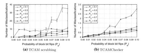
Fig. 4 Comparison of TCAM scrubbing and TCAMChecker for block errors while varying values of  $P_S$ ,  $P_C$  and  $P_e$ . The results are reported for a filter set with 136 rules and the accompanying network trace containing approximately 136 thousand packet headers
