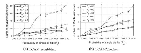
Fig. 3 Comparison of TCAM scrubbing and TCAMChecker for single bit errors while varying values of  $P_S$ ,  $P_C$  and  $P_e$ . The results are reported for a filter set with 136 rules and the accompanying network trace containing approximately 136 thousand packet headers
