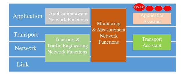
Fig. 5. Classes of advanced functions of FlexNGIA and their operating layers. The figure shows also two special network functions proposed in FlexNGIA (i.e., Application assistant and Transport Assistant)
