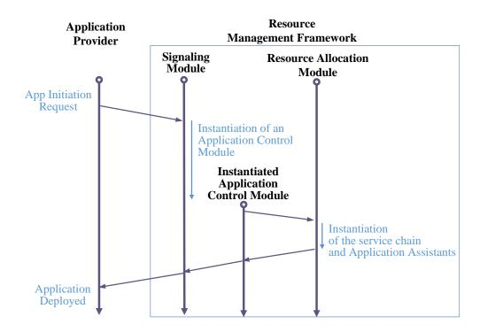
Fig. 10. Signaling - application instantiation process
