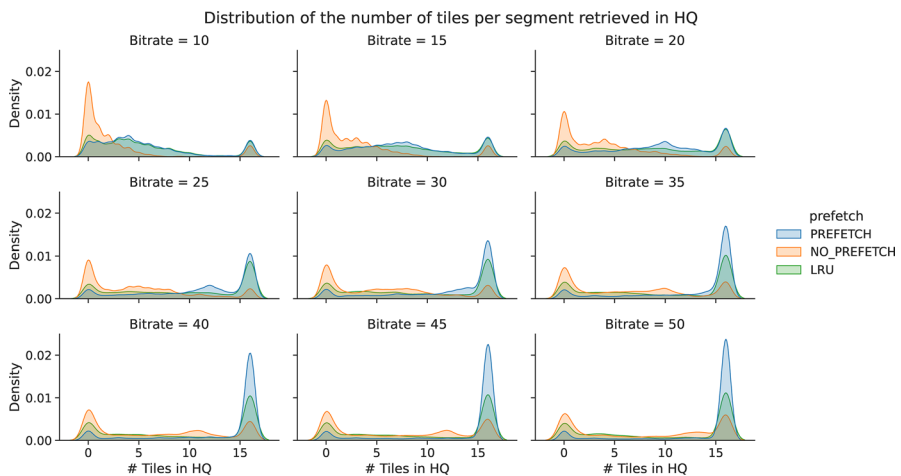
Fig. 14 Distribution of the number of HQ tiles per segment: In comparison to the LRU and NO_PREFETCH configurations, the number of tiles retrieved in HQ from the prefetch setup increases more rapidly as the bandwidth grows larger. Bitrate values in the charts are in Mbps
