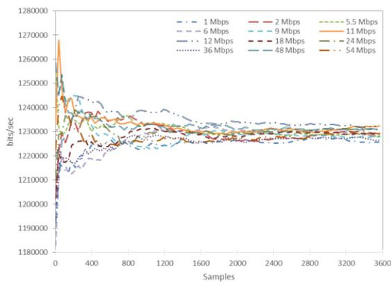
Figure 7. Traffic injected in each IEEE 802.11b/g PHY-mode with a packet size of 1024 bytes.
