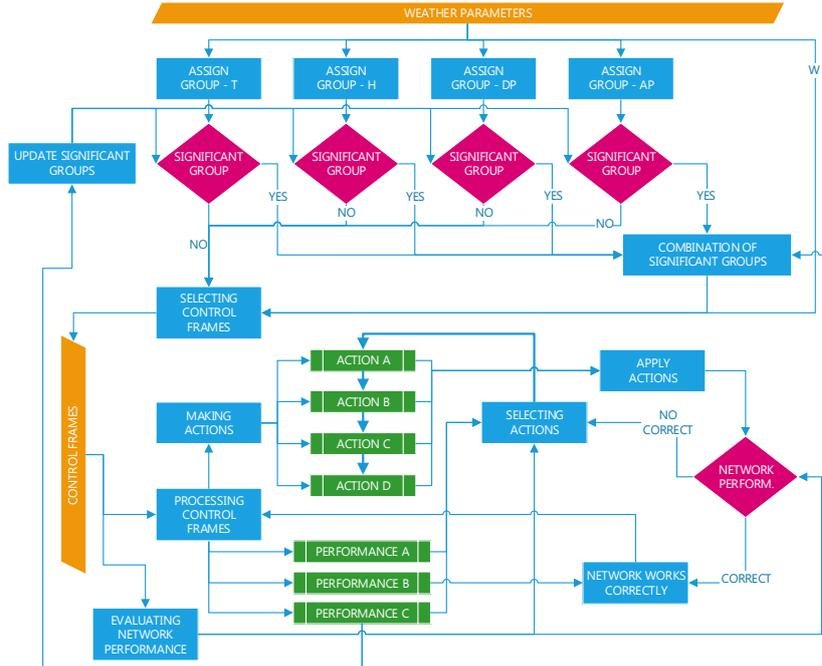
Figure 7. Detailed scheme of green cognitive module.
