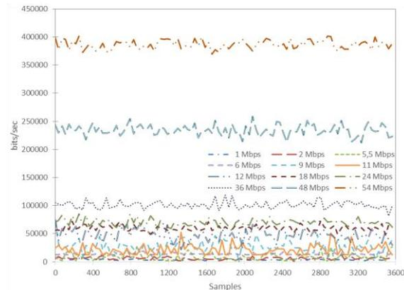
Figure 8. Data dropped by retry threshold exceeded in each IEEE 802.11b/g PHY-mode.
