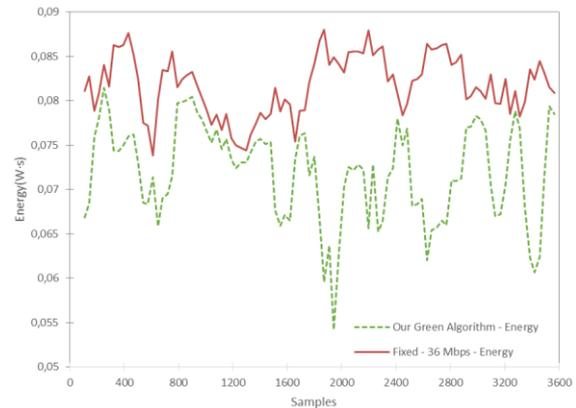
Figure 13. Comparison of energy required in 36 Mbps for a wireless station.
