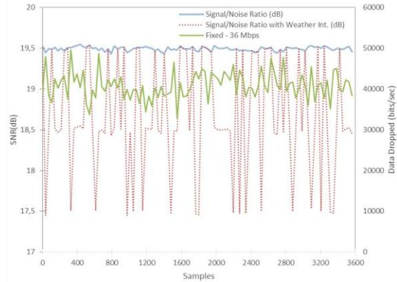
Figure 11. SNR vs. data dropped by retry threshold exceeded in 36 Mbps for a wireless station.
