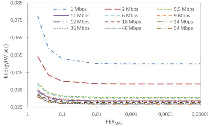
Figure 4. Energy consumption versus frame error rate at MAC layer according to data rates
