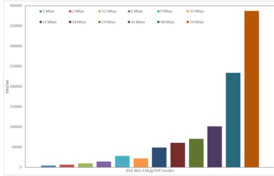
Figure 9: Data dropped on average by retry threshold exceeded in each IEEE 802.11b/g PHY-mode
