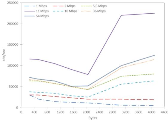
Figure 10. Data packet size variation vs. control traffic introduced for a wireless station in several IEEE 802.11b/g PHY-mode.
