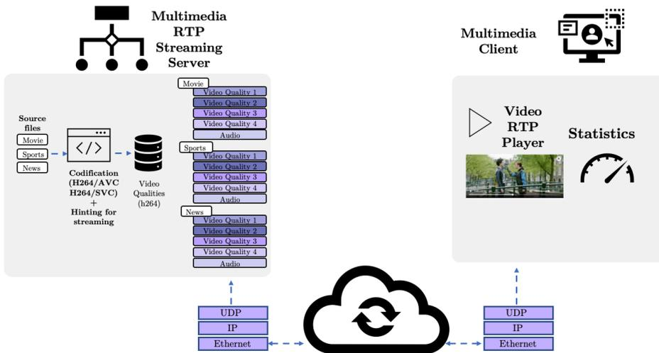
Figure 4.1 IPTV streaming service testbed
