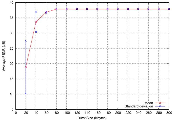
Figure 3.11 Average PSNR and standard deviation, 10 video flows.
