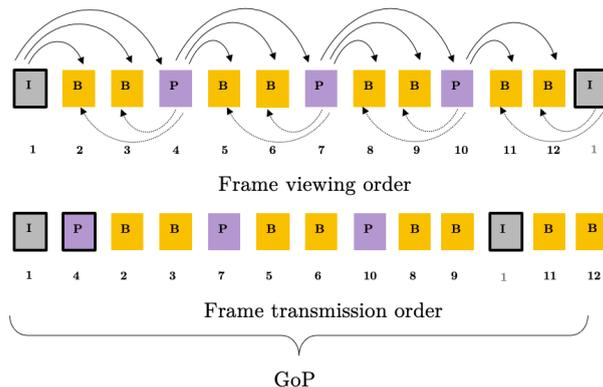
Figure 2.1 Compressed video frame sequence
