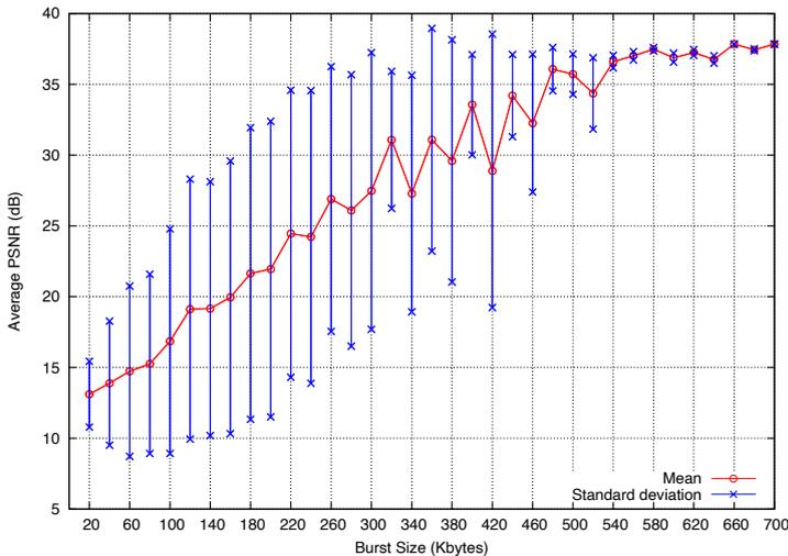
Figure 3.13 Average PSNR and standard deviation, 100 video flows
