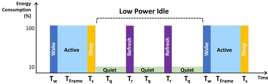
Figure 4.3 Energy consumption and time periods in high and low power modes in 802.3az
