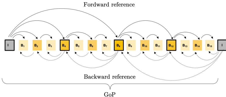
Figure 2.2 Compressed video frame sequence in H.264/SVC
