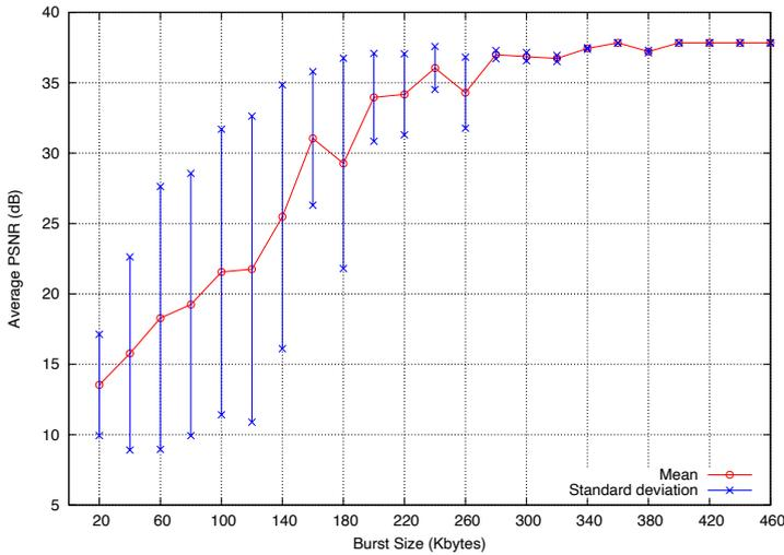
Figure 3.12 Average PSNR and standard deviation, 50 video flows
