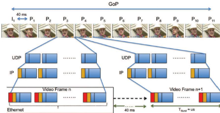
Figure 4.2 Top-down video frame packetization
