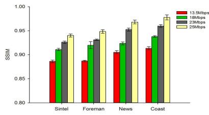
**Fig. 7** Video quality after transmission over IEEE 802.11ad link for 4K UHD video compressed by HEVC at various bitrates (PLR approx. 0.1). Notice the truncated vertical scale.
