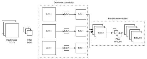
Fig. 2 Illustration of the working of a depthwise separable convolution network
