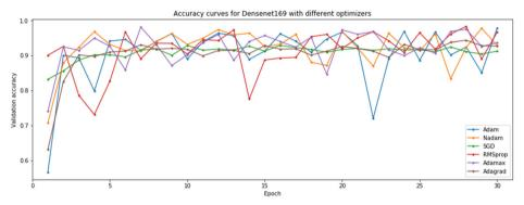
Fig. 11 Densenet169 model performance on the validation set using different optimizers
