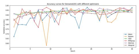
Fig. 12 Densenet201 model performance on the validation set using different optimizers
