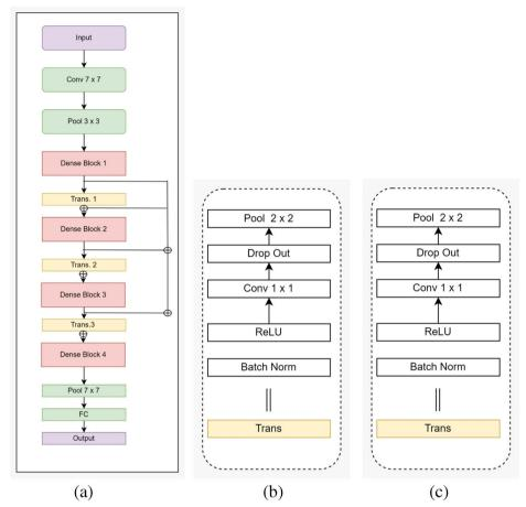
Fig. 4 a The entire architecture of DenseNet deconstructed into in b Trans block with Dense interconnections and c Dense block used in the DenseNet architecture
