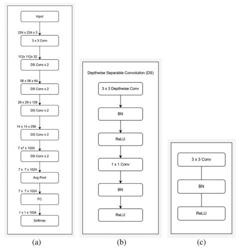
Fig. 3 a Entire MobileNet architecture with normal convolutions and depthwise separable convolutions. b All the layers following a depthwise separable convolution block. c All the layers following a normal  $(3 \times 3)$  convolution block in MobileNet architecture
