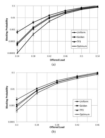
**Fig. 7.** Bandwidth Blocking Probability versus Offered Load for the different traffic profiles considered. Multi-Rate connections are generated. (a) NSFNet topology. (b) US\_Backbone topology.
