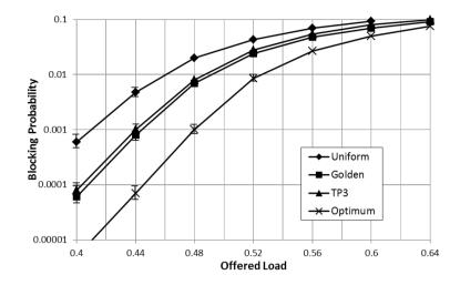
Fig. 4. NSFnet network Blocking probability (BP) versus Offered Load for the different traffic profiles considered. Elastic (1 to 10 FS) connections are generated.
