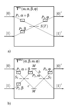
FIG. 1: A universal quantum interference device operating on a qubit can be realized by a 4-port interferometer with two input ports  $|0\rangle, |1\rangle$  and two output ports  $|0\rangle', |1\rangle'$ ; a) realization by a single beam splitter S(T) with variable transmission T and three phase shifters  $P_1, P_2, P_3$ ; b) realization by two 50:50 beam splitters  $S_1$  and  $S_2$  and four phase shifters  $P_1, P_2, P_3, P_4$ .
