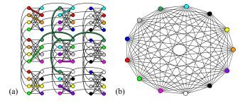
FIG. 2. [Color online] Example of embedding  $K_{13}$  in the Chimera(3,3,4) virtual hardware construction: (a) the embedding of a logical qubit into 6 physical qubits is highlighted (dark green), (b) of the 13 vertices on  $K_{13}$ , 11 are chains of order 6 (various colors) while 2 are chains of order 3 (black)
