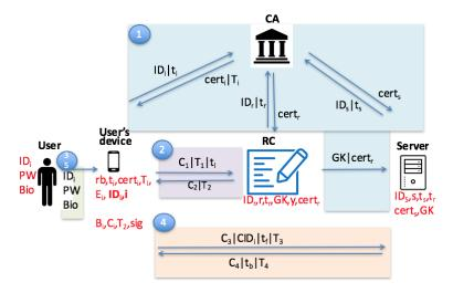
Fig. 3: Steps and computations during the registration request of user with RC
