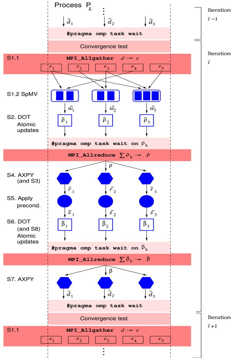
Fig. 4 Dependencies between kernels in the BJCG solver.
