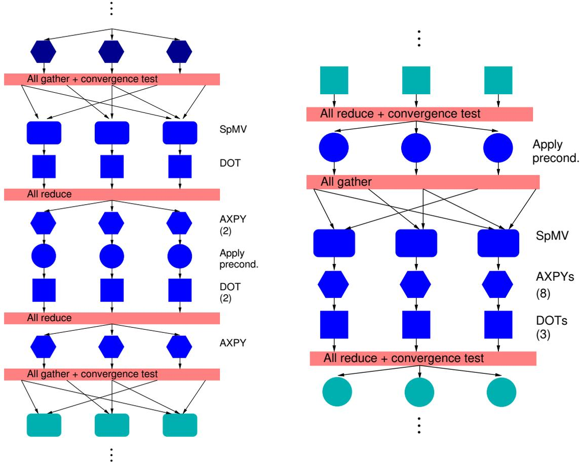
**Fig. 7** Simplified dependencies between kernels in the classical BJCG solver and the pipelined variant (left and right, respectively). In both cases, a single iteration comprising the operations/kernels between two consecutive convergence tests is shown.
