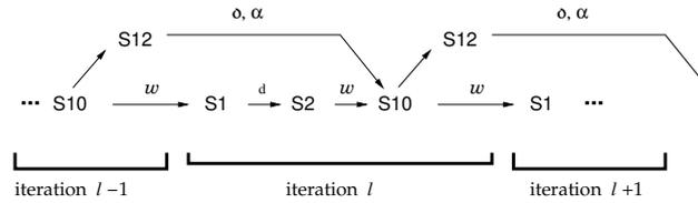
**Fig. 6** TDG of the dependency pattern in the task-parallel pipelined BJCG solver.
