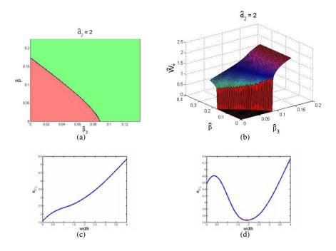
Fig. 4.  $\hat{d}_2=2<\hat{D}_2$ . (a): different regions in the  $\hat{\beta}_3-\hat{\beta}$  plane.  $e_{P,L}$  has either no local minimum (red) or one local minimum (green). (b): the associated stable bar width  $\hat{W}_*$ . (c):  $e_{P,L}$  with no local minimum ( $\hat{\beta}=0.05, \hat{\beta}_3=0.04$ ). (d):  $e_{P,L}$  with one local minimum ( $\hat{\beta}=0.2, \hat{\beta}_3=0.1$ )
