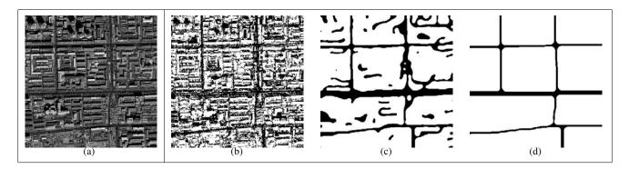
Fig. 8. Data, and experiment at 1/4 resolution. (a): image data (size  $=350\times350$ , road width  $=3\sim5$  pixels). (b)-(d): results obtained using the new nonlinear model (with  $E_{NL}$ ) at iterations 1, 1,500 and 27,000
