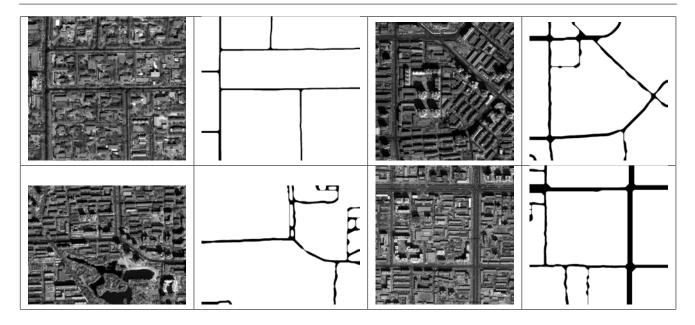
Fig. 13. More results using the new linear model (with  $E_L$ ) on pieces of a QuickBird image at full resolution. Image size: top left:  $800 \times 880$ ; top right:  $1200 \times 1200$ ; bottom left:  $1200 \times 1600$ ; bottom right:  $1400 \times 1400$
