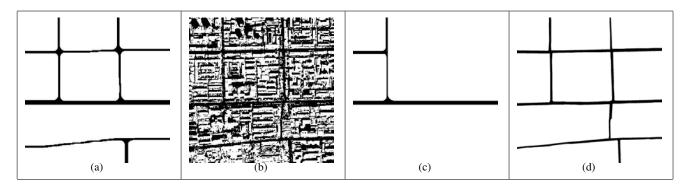
Fig. 9. Experiments at 1/4 resolution and ground truth. (a)-(c): results obtained respectively using the standard energy without  $E_{NL}$ , MLE, and a standard, non-higher-order active contour model (with neither  $E_S$  nor  $E_{NL}$ ). (d): ground truth segmented manually
