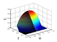
Fig. 3. Diagram of the scaled control parameters  $\hat{\beta}$  and  $\hat{\beta}_2$ , and the scaled width  $\hat{W}$ , when w=2. The left part of the surface represents the parameter space for which  $e_{P,NL}$  has one local maximum; in the right part of the surface,  $e_{P,NL}$  has one local minimum; and the borderline between them, where  $\hat{W}=0.8798$ , represents the situation when two extrema become an inflection point
