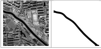
Fig. 14. Result of river extraction on a QuickBird panchromatic image (size:  $1024 \times 1024$ )
