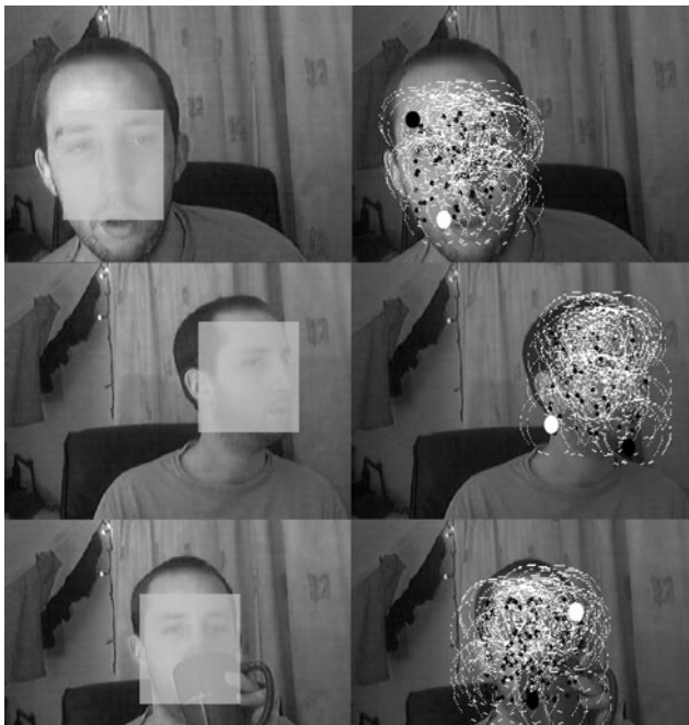
Fig. 21 The medoidshift algorithm tracks the head sequence ( top row ). LP positions ( small black dots ) and support pixel ranges ( white dashed circles ) are shown as well as the worst predictor from the current frame ( large black circle ) and the predictor learnt from this frame ( large white circle ). It is this process that generates view-specific displacement predictors within the model
