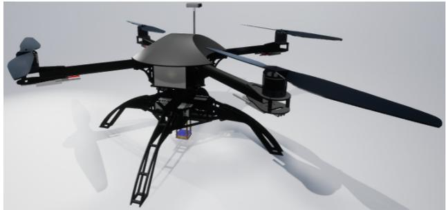
Fig. 2: The tracking UAV rendered inside Sim4CV. The UAV is equipped with gimballed landing gear allowing for both a stabilized camera and articulated legs for gripping of objects in multi-agent simulation tasks.
