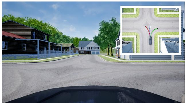
Fig. 16: An example showing results of our guided driving method. The car is located at an intersection. The image in the top right corner shows the situation from above with a visualization of the waypoint predictions when the goal input is set to  $-1$  (red/left),  $0$  (blue/straight) and  $1$  (green/right), respectively.
