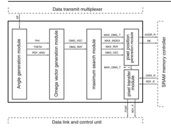
**Figure 15** Image processing and application unit block diagram. For the sake of clarity, only the pertaining sub-blocks for omnidirection vision construction are shown.
