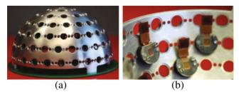
**Figure 3 a** Side view, **b** and internal view of the fabricated Panoptic camera with individual imagers.
