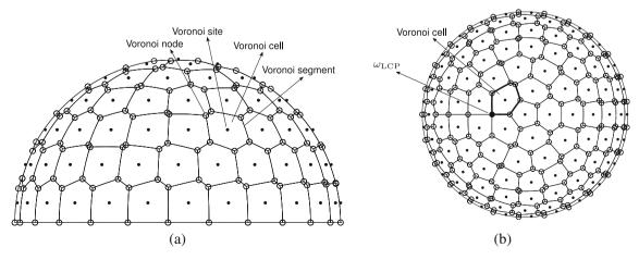
Figure 7 a Side view of the Voronoi diagram of the pixelized hemispherical structure with seven floors, b top view of the Voronoi diagram of the same structure.
