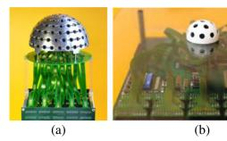
**Figure 18** The built setup of FPGA platforms for Panoptic systems with, a 7-floor and 13 cm diameter hemisphere structure with thirty embedded cameras, **b** 3-floor and 3 cm diameter hemisphere structure with fifteen embedded cameras.
