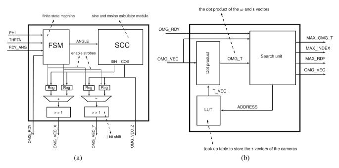
Figure 16 a Internal architecture of the omega vector generation module with one sine and cosine calculator module; b the nearest camera position finder module.
