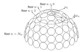
Figure 1 Hemispherical structure with six floors.
