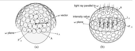
The projected points of the contributing camera positions in  $\omega$  onto the  $\omega$  are highlighted by hollow points in Fig. 6a and b. Following the CLF assumption, each projected camera position  $P_{c_i}$  on the planar surface is assigned an intensity value  $\mathcal{L}(\mathbf{c}_i, \omega)$  (Fig. 6b).
