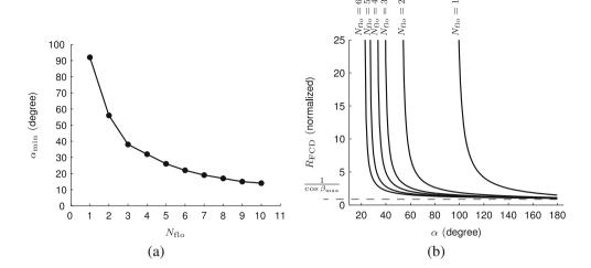
The full-view coverage distance  $R_{\rm FCD}$  for several Panoptic devices with  $N_{\rm flo}+1$  latitude floors versus the AOV of the cameras are depicted in Fig. 9b. As the number of latitude floors increase and hence the number of cameras, identical full-view coverage distance is reached at smaller AOVs. A similar trend is observed for all Panoptic devices, as the AOV of their cameras increase their full-view coverage distance decrease.
