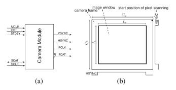
Figure 11 a Camera module interface, b camera frame.
