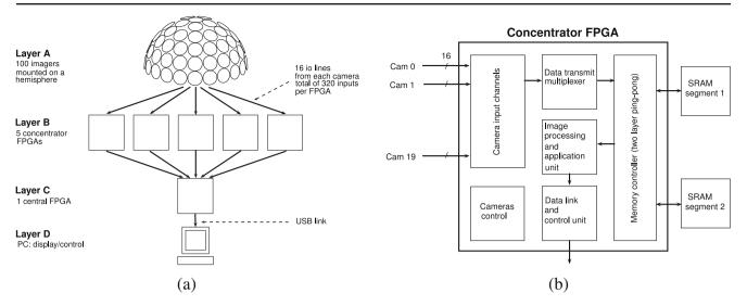
Figure 10 a Architecture of the full hardware system and, b architecture of a concentrator FPGA.
