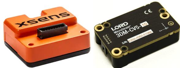
Fig. 3: Commercial attitude and heading reference systems with built-in IMUs from XSens Technologies BV and LORD MicroStrain, with three accelerometers, three gyroscopes, three magnetometers and three temperature sensors for sensor calibration. These IMUs include coning and sculling compensation (see Section V), which enables them to deliver attitude data at low rates without losing accuracy.
