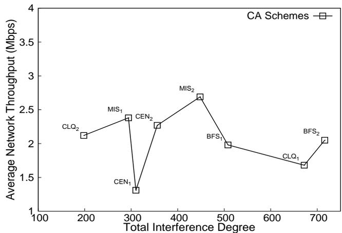
Fig. 16: Correlation of TID with Average  $\text{Throughput}_{Net}$
