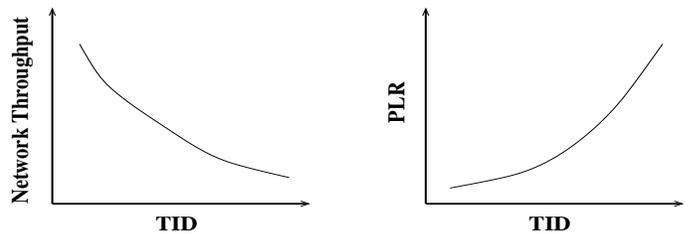
Fig. 15: Expected correlation of TID with  $\text{Throughput}_{Net}$  and PLR
