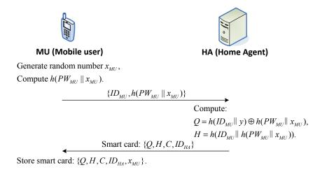
Figure 4: Registration phase of the proposed scheme.
