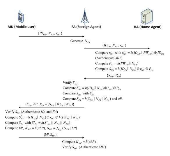
Figure 2: Authentication and establishment of session key phase of Mun et al.'s scheme.
