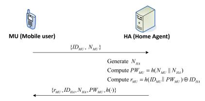
Figure 1: Registration phase of Mun et al.'s scheme.
