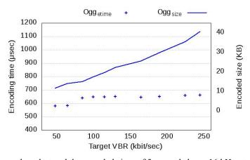
Fig. 6. Processing times on the robot and the encoded sizes of 3-seconds long, 16 kHz, stereo audio chunk with Ogg codec. The results are shown in the function of the target VBR bitrate. The crosses are related to the left scale, the lines to the right scale.
