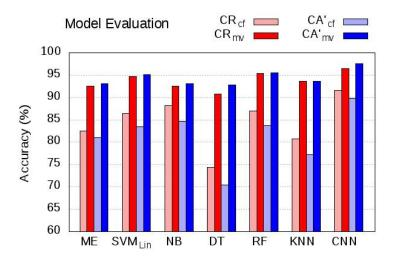
Fig. 3. Model evaluation of seven classifiers over the validation set  $(CR_V)$  of CSIBE-RAW (red) and CA'<sub>V</sub> of CSIBE-AIBO (blue). The lighter colors (odd columns) were the aggregated frame-based evaluations and majority voting was used in the darker (even columns) in addition.
