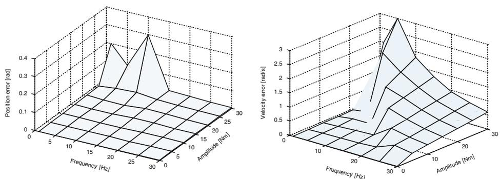
disturbances varied from 0 to 30 Hz with amplitudes varying from 0 to 30 Nm, and the disturbances have been injected at the would point where the user exercises forces onto the robot. For this simulation, the saturation of the motors has been set to 25 Nm.
