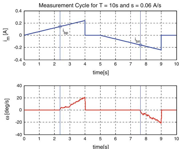
**Fig. 2** Breakaway friction identification procedure for Configuration 2 with the parameters  $s = 0.06$  A/s and  $T = 10$  s. The graph shows the motor current  $i_m$  and the angular velocity  $\omega$ . The vertical lines indicate the point in time when the rotor starts to turn ( $t_{bp} \approx 2.35$  s,  $t_{bn} \approx 7.6$  s) and when the breakaway currents  $i_{bp}$  and  $i_{bn}$  are captured. This procedure is repeated 200 times for each configuration
