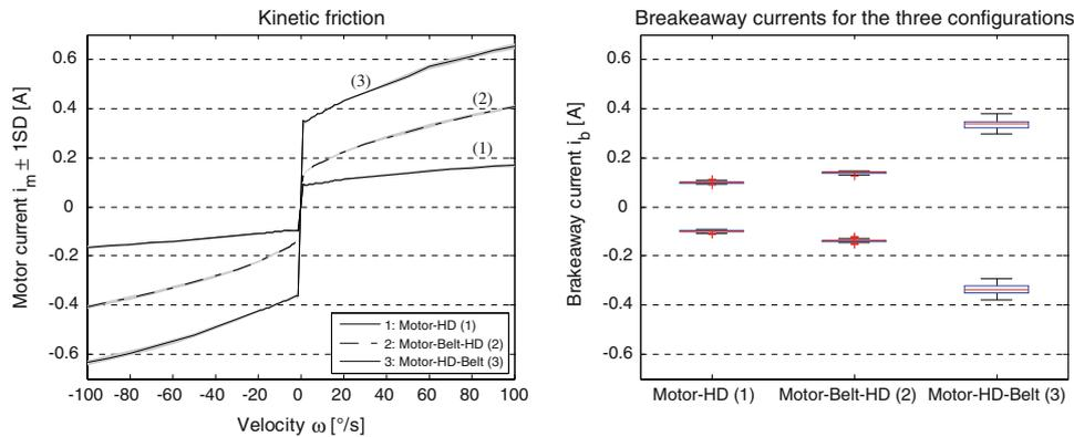
**Fig. 4** Kinetic and breakaway friction for the three configurations. The kinetic friction has been identified by measuring the motor current  $i_m$  that is required to drive the motor at the given velocity  $\omega$ . To determine the breakaway friction, a slow current ramp has been
