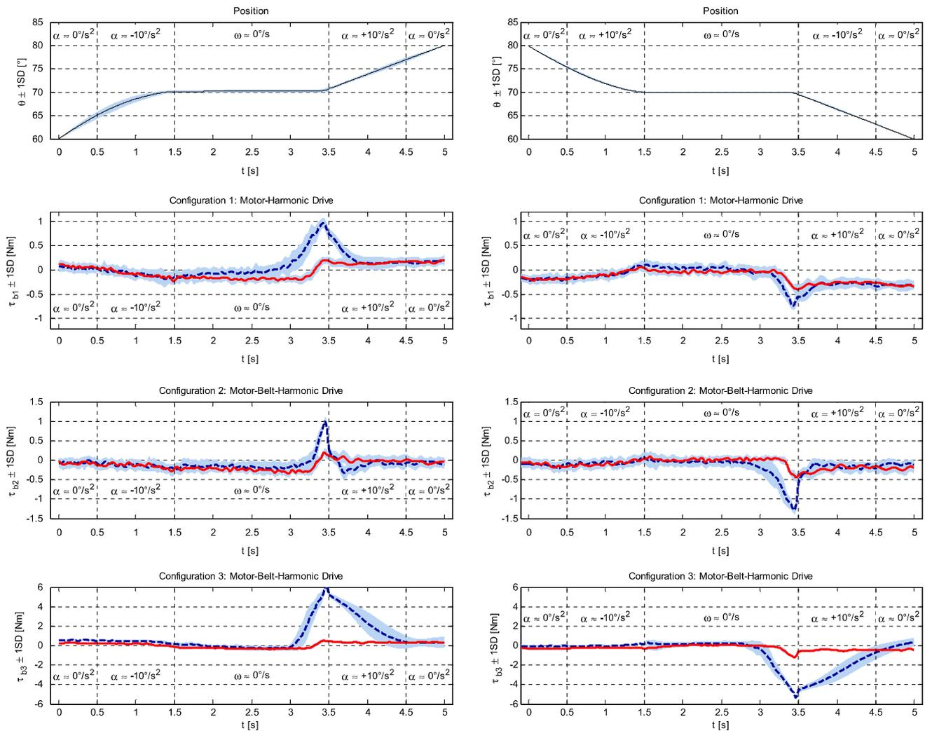
**Fig. 5** Results of the experimental evaluation. All lines represent the average and standard deviation of ten movements. The first row shows the trajectories and the other plots show the interaction torque
