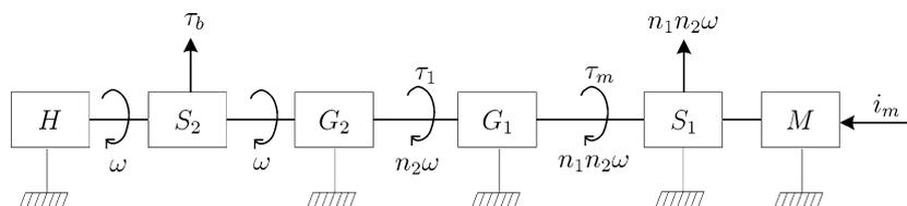
**Fig. 1** Experimental setup with DC motor  $M$  (RE 35, Maxon Inc.), incremental position encoder  $S_1$  (4000 imp/rot), gearbox  $G_1$  with the reduction ratio  $n_1$ , gearbox  $G_2$  with the ratio  $n_2$ , torque sensor  $S_2$  (6
