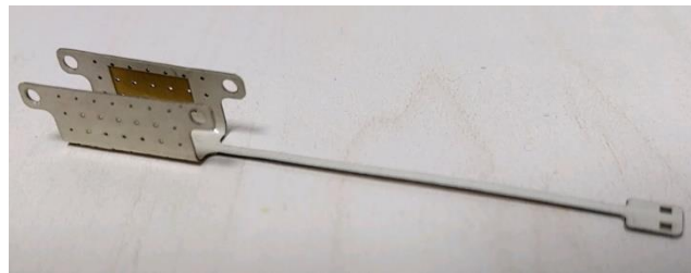
Fig 3. Fabricated LCP outer box with gold electrode and macro and micro holes: four macro holes are at the edge of the outer box to fix the device with screws at the bone defect. Micro holes are at the surfaces of the outer box to facilitate flow of body fluids between in and out of the box. Two gold electrodes are located at the side walls of the box for electric stimulation
