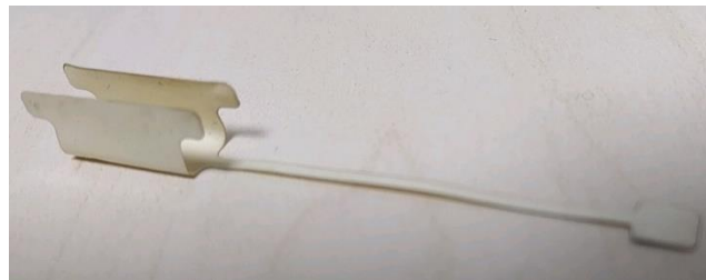
Fig 2. Fabricated LCP outer box whose shape and size are tailored to the target bone defect: the structure of the outer box is half cylindrical shell whose cross-section is U-shape. Size of the outer box is 15 mm in length, 7 mm in height, 6 mm in width. Thickness of the shell is 0.35 mm and interconnection line of 5 cm-length is extended for connection to electric stimulator
