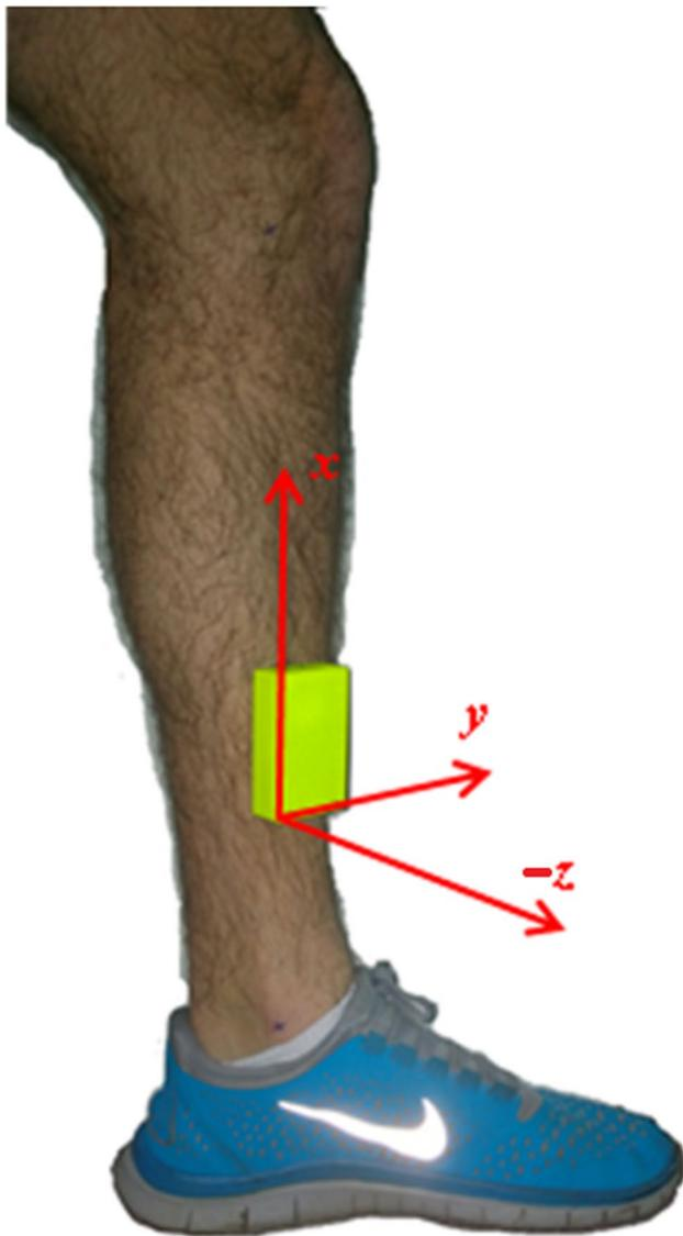
**Fig. 1** Tibial accelerometer. Axes;  $x$ =along-tibial axis,  $y$ =perpendicular to  $x$  along to second edge of the sensor casing and,  $z$ =perpendicular to  $x$  along the short edge of the sensor casing
