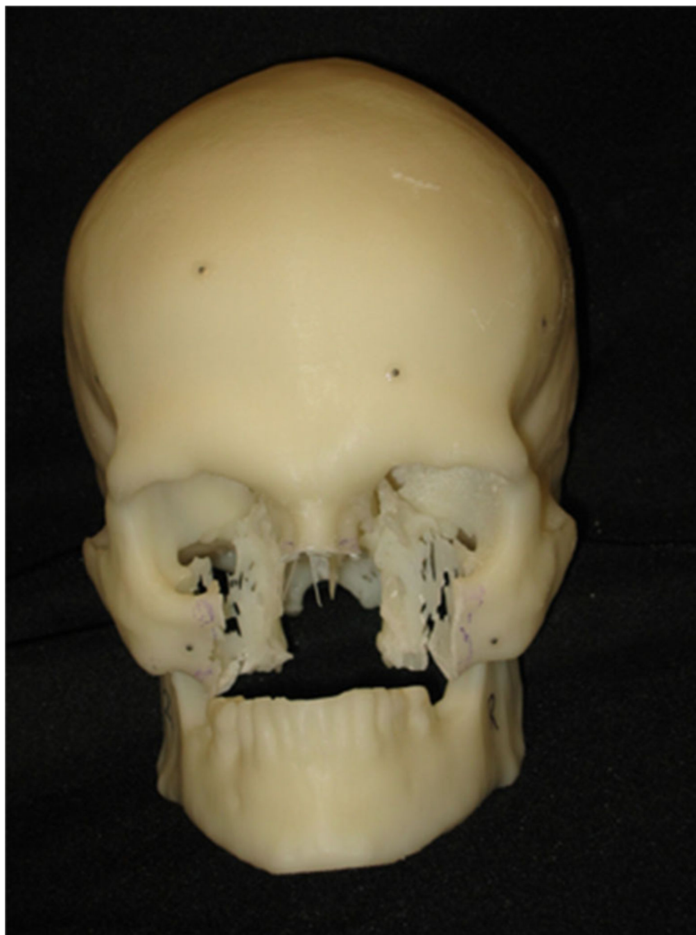
Fig. 6. Printed plastic human skull (recipient) with fiducials attached and simulated trauma
