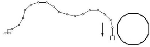
Fig. 2 End-effector motion of a planar hyper-redundant manipulator
