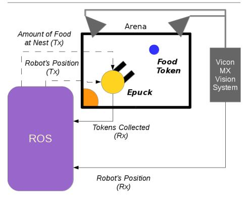
Fig. 7 Main data flows of the real-robot experiment setup. The use of the Vicon MX tracking system and ROS infrastructure were two important features of the experimental setup, needed to provide the robots with virtual sensing of the nest and amount of food collected. Tx refers to ROS topics that were used in order to send information from the ROS main instance into the robots. Rx refers to ROS topics used in order to receive information from the environment and robots into the ROS system.
