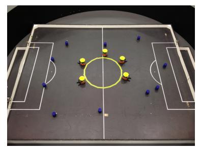
Fig. 5 Photo of the arena used in order to conduct the real-robot experiments. In the picture, five e-puck robots (in *Wait* action) gather in the middle of the experiment space, surrounding the nest (circle located at the center), and 10 food tokens are scattered in the arena. Note that the other markings in the experimental arena have no significance
