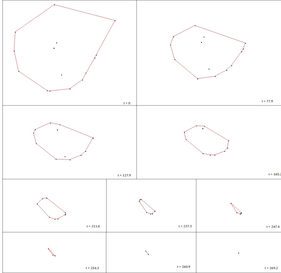
Figure 7: Configuration of the swarm at different times. The convex hull of the set of agents is also shown.
