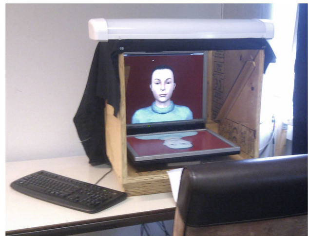
Fig. 3 Experiment setup at speaker side. The setup at the listener’s side is similar, but displays the video of the speaker instead of a virtual representation. A camera is placed behind the one-way mirror
