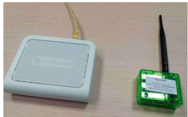
Fig. 8 Indoor gateway used for measurement 3 experiments on the left side and packaged Pycom device on the right side
