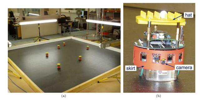
Fig. 1 (a) Artificial culture lab showing 6 robots in the arena. (b) An e-puck with Linux board fitted in between the e-puck motherboard (lower) and the e-puck speaker board (upper). Note both the red skirt, and the yellow 'hat' (which provides a matrix of pins for the reflective spheres which allow the tracking system to identify and track each robot).
