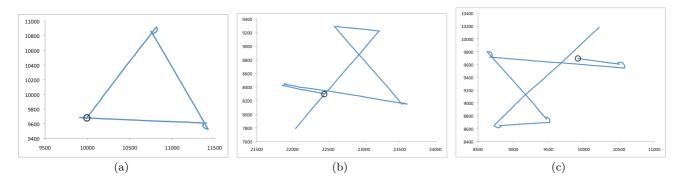
Fig. 5 (a) Meme 1: initial movement meme enacted by e-puck 9. (b) Meme 2: imitation of meme 1 by e-puck 12,  $Q_i = 0.47$ . (c) Meme 3: imitation of meme 2 by e-puck 9,  $Q_i = 0.94$ . X and y axes are labelled in multiples of 0.1 mm and the circles mark the start positions of each movement-meme.
