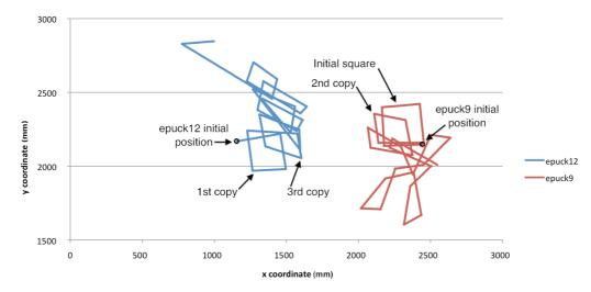
Fig. 3 Trajectory plot: two robot imitation. The experiment starts with e-puck 9 in teacher mode, following a movement trajectory that describes a square with sides of 25cm; e-puck 12 is initialised in learner mode.
