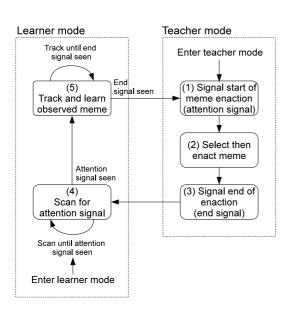
Fig. 2 Finite State Machine for Copybots. Unlabelled transitions take place when the previous state completes (timings are explained in the text). Different entry points for robots starting in teacher or learner modes are shown. Once started the FSM loops indefinitely, alternating between teacher and learner modes.
