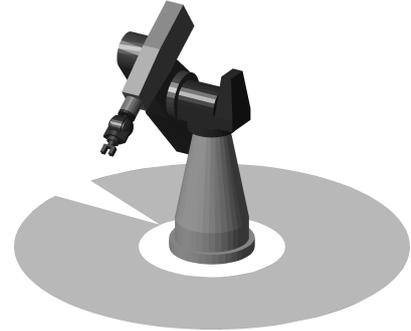
Fig. 6.8: The Puma robot arm with six degrees of freedom.
