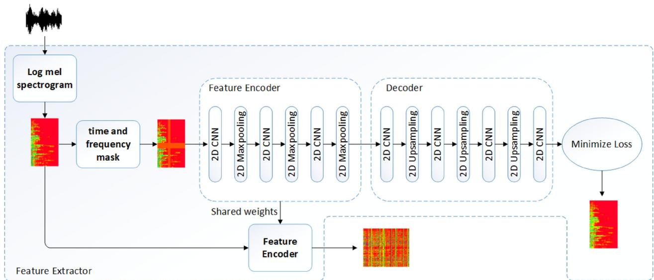
**Fig. 2** Detailed design for feature representation. For each segment-level audio, it is transformed into log-mel spectrogram, followed by frequency and time masking. Then, such input is fed into a CNN-based
