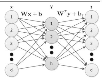
**Fig.1** The structure of an autoencoder where  $\mathbf{x} \in \mathbb{R}^d$  contains the input values,  $\mathbf{y} \in \mathbb{R}^h$  is the hidden representation of the input values,  $\mathbf{z} \in \mathbb{R}^d$  is the reconstruction of the input, **W** is a matrix containing the weight values and **b**,  $\mathbf{b}_{\tau}$  are bias vectors
