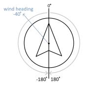
Fig. 3. Wind direction representation. The UAV heading is defined as 0°. If the wind direction is to the left of the UAV heading, it is negative; if it is to the right of the UAV heading, it is positive.
