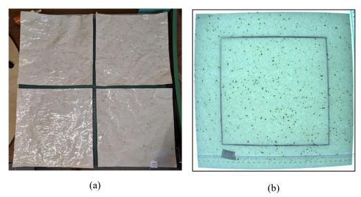
Fig. 8. a) Large sample was cut into four smaller sample squares. b) Each smaller sample square was imaged individually on a light board. The vermiculite showed up as dark dots in contrast to the background when placed on a light table.
