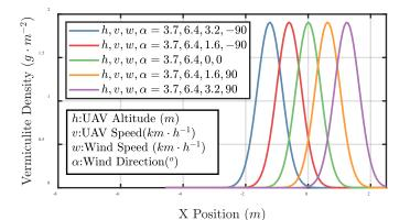
Fig. 17. The combined effects of wind speed and direction on vermiculite distribution. The areas under the blue, red, green, orange, and purple curves (in g  $m^{-1}$ ) are the same, which is 574.
