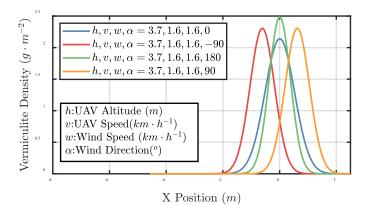
Fig. 16. The effects of wind direction on vermiculite distribution. The areas under the blue, red, green, and orange curves (in g m<sup>-1</sup>) are 850, 759, 714, and 759, respectively.
