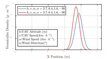
Fig. 18. The effects of UAV altitude on vermiculite distribution, during a lateral wind. The areas under the blue and red curves (in g  $m^{-1}$ ) are 548 and 575, respectively.
