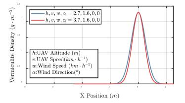
Fig. 14. The effects of UAV altitude on vermiculite distribution, when there is no wind. The areas under the blue and red curves (in g  $m^{-1}$ ) are 879 and 759, respectively.
