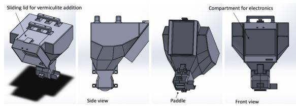
Fig. 4. CAD drawing of our Bugbot dispenser design.
