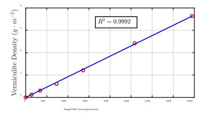
Fig. 9. Linear regression curve for the conversion of imaged dark area (in square pixels) to vermiculite density (in g m<sup>-2</sup>). The calibration equation is *Vermiculite Density* =  $0.0428 \times Imaged Dark Area$ .
