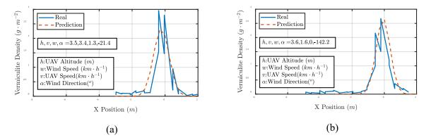
Fig. 13. Comparison of real vermiculite density data and density predicted by our mathematical model. The learned functions of the Gaussian coefficients (see Eq. (4)) are as follows:
