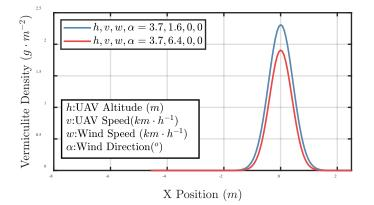
Fig. 15. The effects of UAV speed on vermiculite distribution, with no wind. The areas under the blue and red curves (in g  $m^{-1}$ ) are 759 and 574, respectively.
