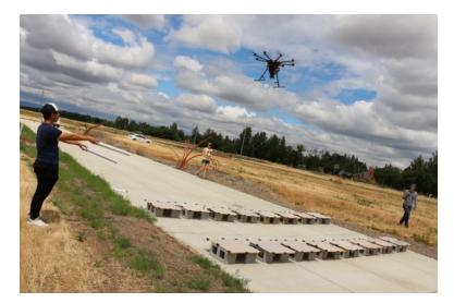
Fig. 7. Procedure taken to correct for GPS error. A timestamp and a visual cue were recorded when the UAV reached a row of boards.
