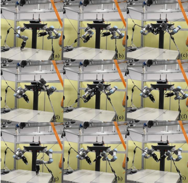
**Fig. 8** The planned motion in real execution. The subfigures (a)-(h) corresponds exactly to the motion planned in the simulation. Subfigure (i) shows the final state after applying compliant control.
