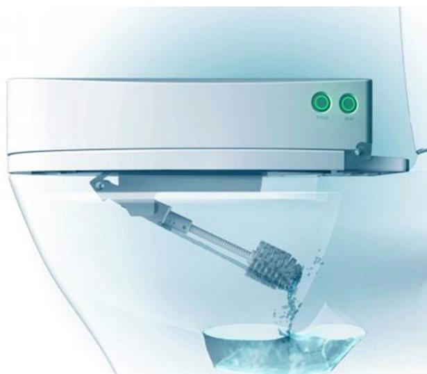
**Fig. 10** SpinX toilet cleaning robot attached to a toilet bowl; Image Courtesy: SpinX Robotics, Inc
