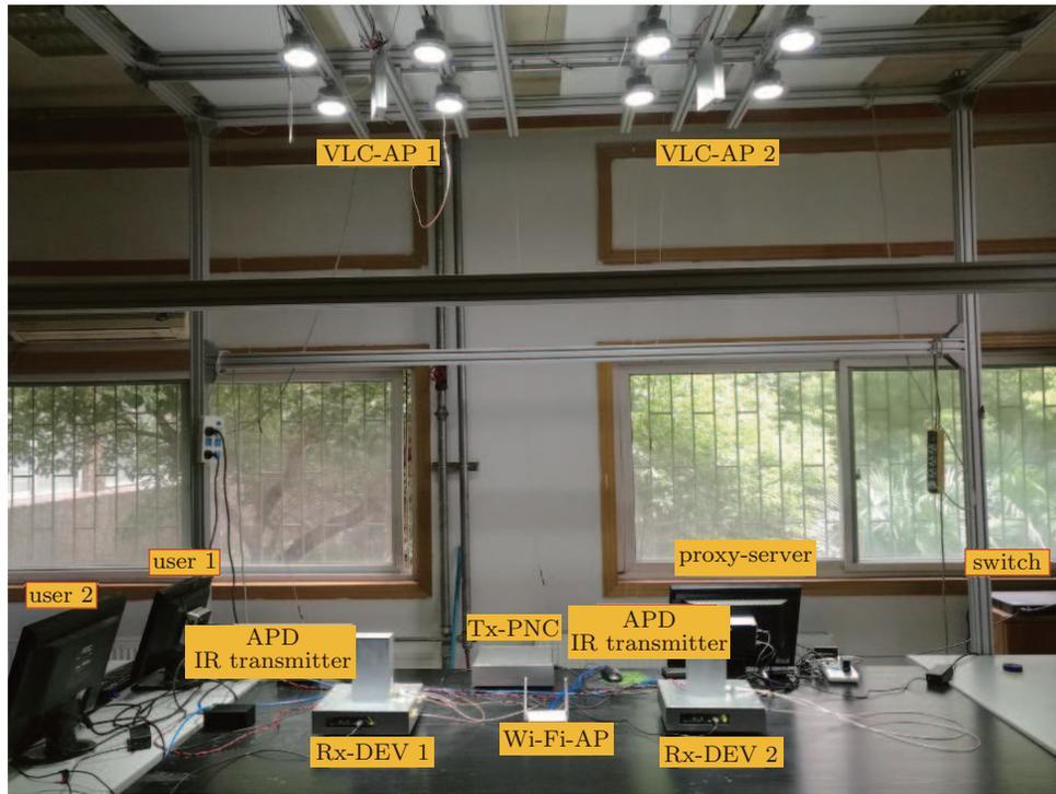
Figure 8 Hybrid VLC-Wi-Fi experiment platform
