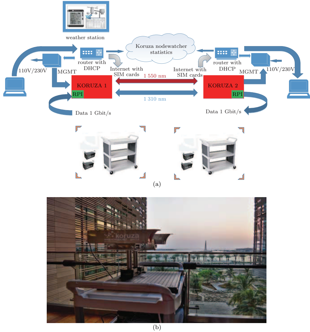
Figure 2 Proposed mobile FSO system: (a) system design; (b) coastal environment
