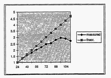
The results are very satisfactory up to about 64 processors and then start to deteriorate. Beginning with 96 processors there is no increase in the speedup nymore. The main reason for this retardation is the fact that the load balancing
