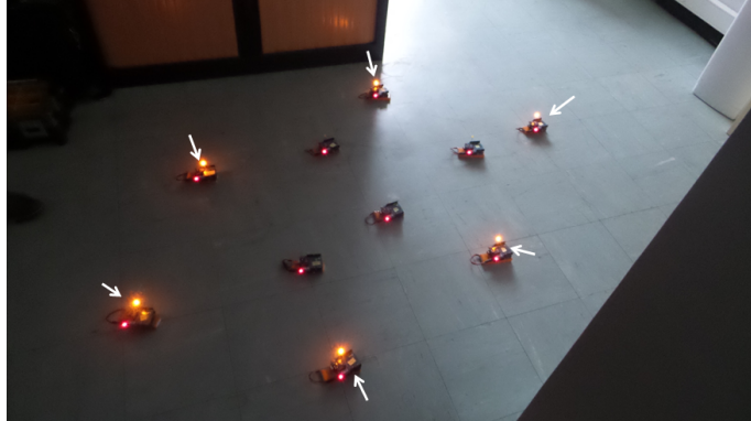
Figure 8: Execution of D-LPCN using real Arduino/XBee sensor nodes.
