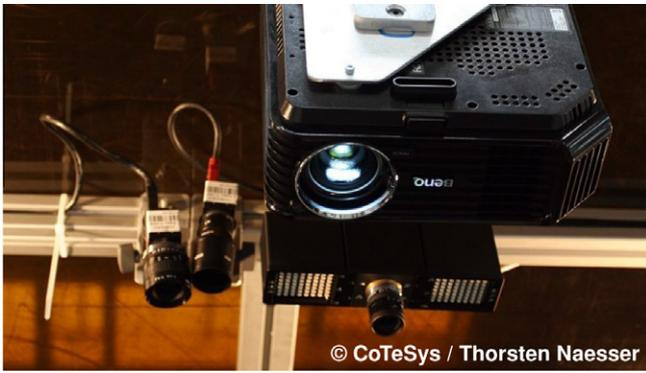
Fig. 2. Sensing devices and a projection unit: two video-cameras, a Phonic Mixer Device camera (PMD) (back, left to right) and a video projector (front).
