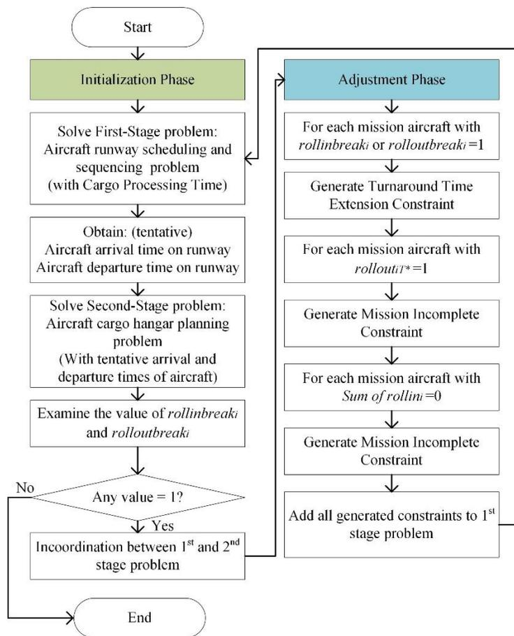
**Figure 6** Algorithmic framework of the two-stage optimization method
