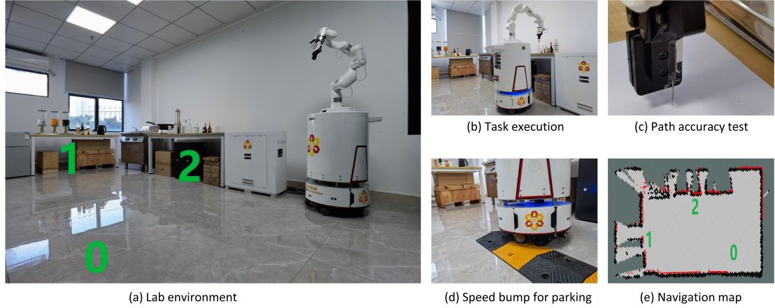
Figure 6: Experiment configuration. (a) shows the experiment environment. The mobile manipulator will conduct experiments at site 0, site 1, site 2, site 2' (site 2 and site 2' are in the same location). (b) shows the robot executing a task. (c) shows the executed path's accuracy test using a needle. (d) shows a speed bump installed at the parking place to emulate uneven terrain. (e) shows the pre-built map for robot navigation. The black lines or dots in the occupancy map represent obstacles ("occupied"). The red lines or dots represent the laser scan which is used for localization. '0', '1' and '2' represent site 0, site 1 and site 2.
